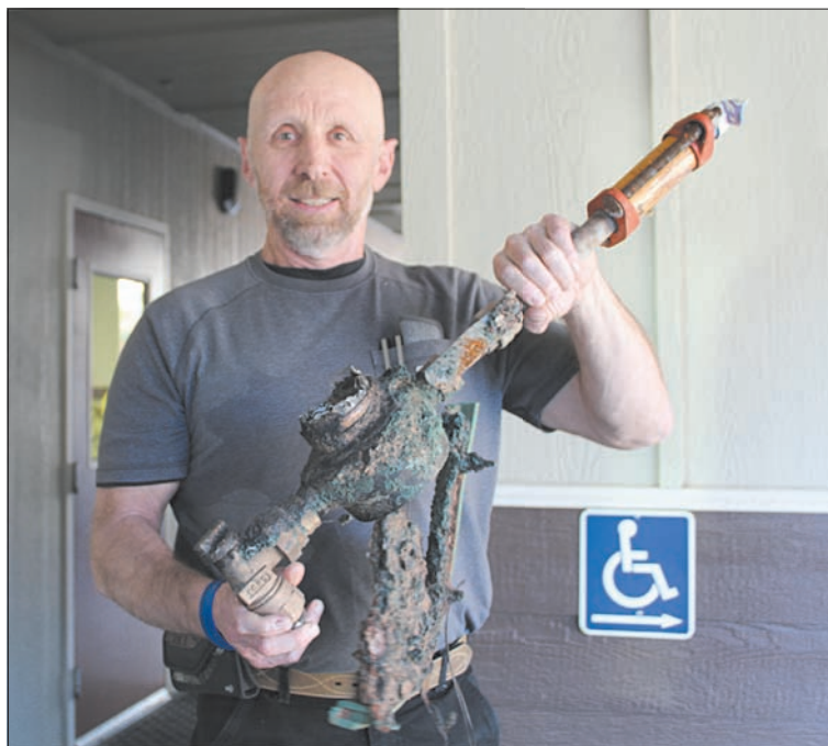
Jim Ladrini, assistant field superintendent for the PID, with a melted water meter. Almost all of the district's meters melted during the Camp Fire, as they—and the boxes and lids that protect them—are made of plastic. They will be replaced with concrete ones.
