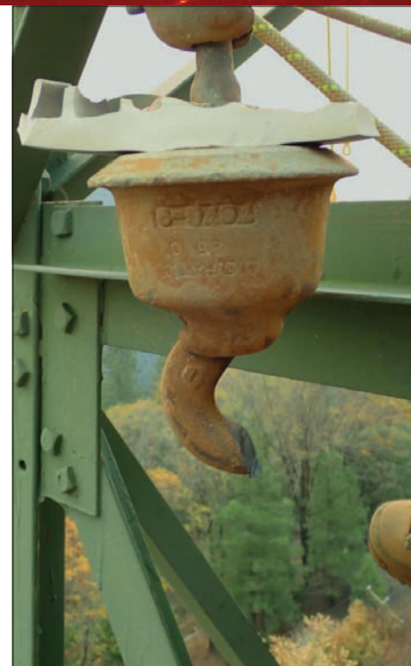
The 2018 Camp Fire, the deadliest and most destructive fire in California history, was caused by a PG&E high-voltage line that busted out of a faulty steel C-hook.
